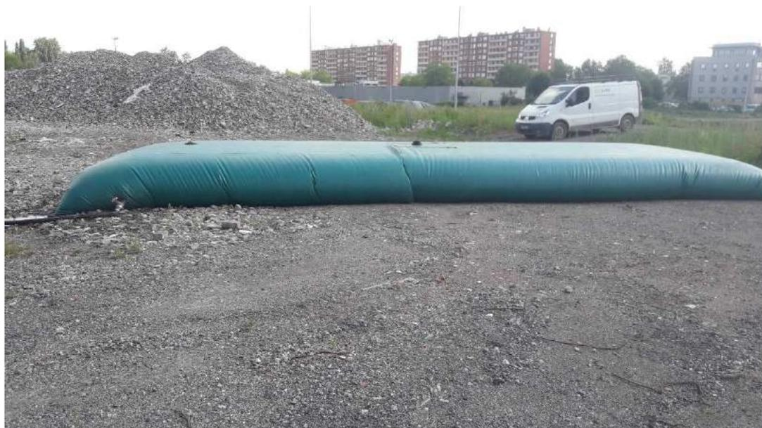
**Photo 11: Cuve souple de stockage**
